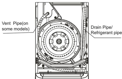
Pipe hole position on both sides
