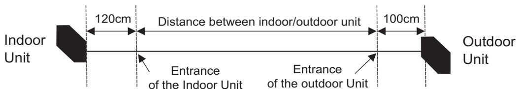
● **Connect the cable between the outdoor unit**
